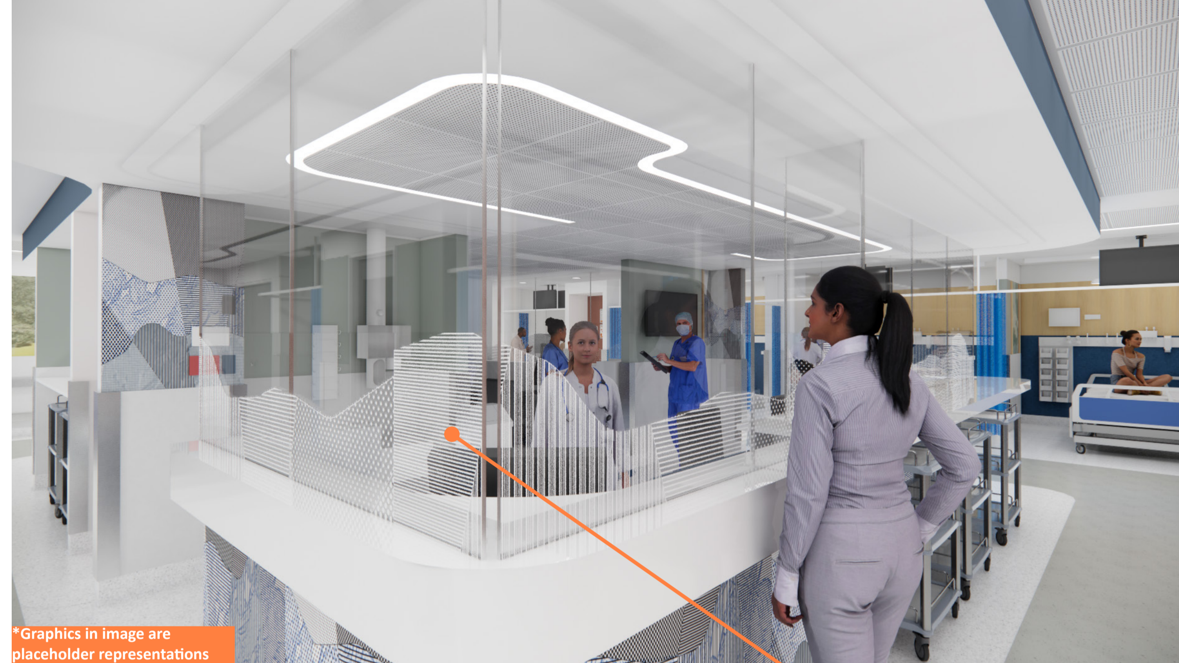
DCLa_G Adhesive glazing film with custom decal. +400mm from bottom of glazing.
