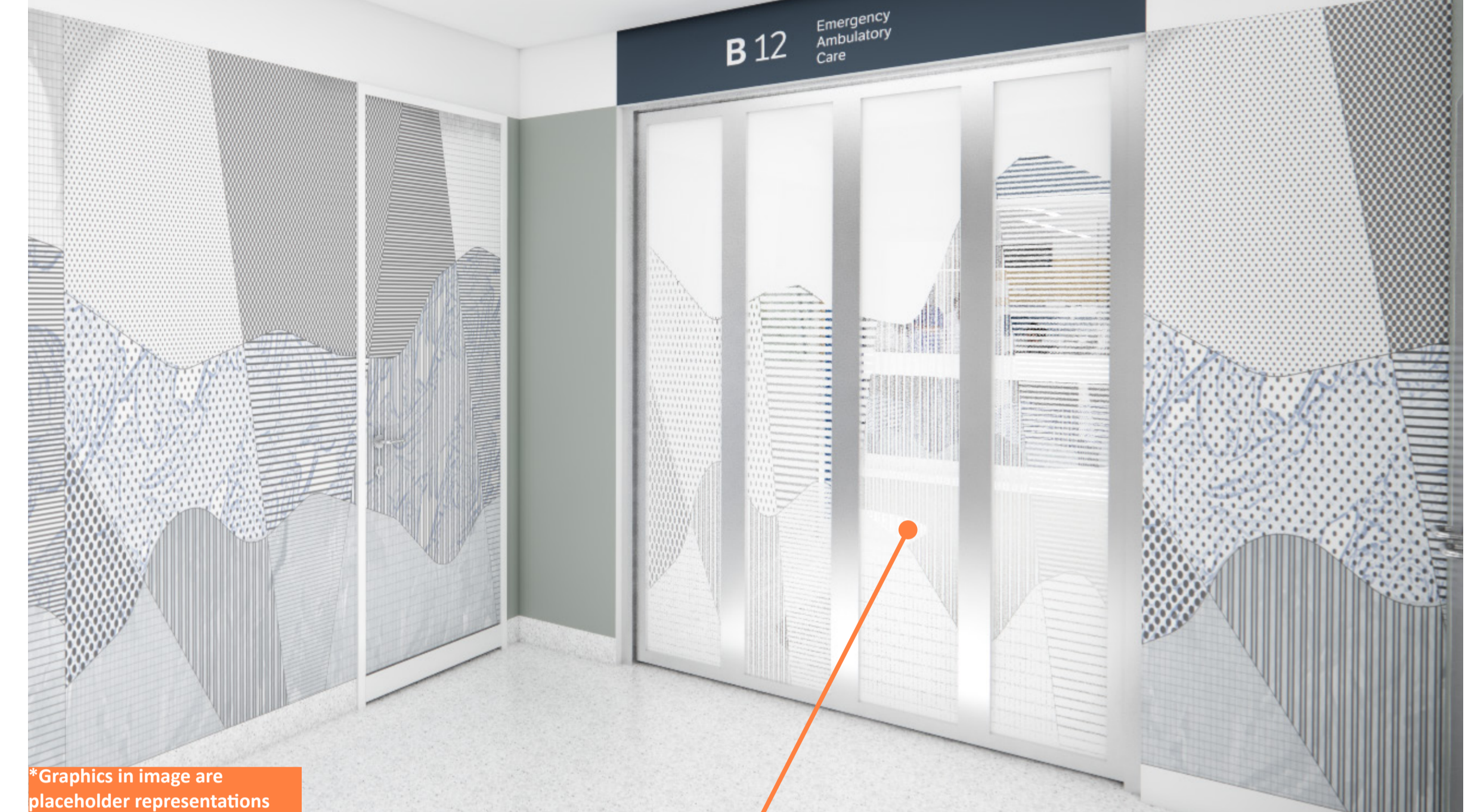
DCLb_G Adhesive glazing film with custom decal to full height of EAC entry doors. 1700x2300mm (wxh).
